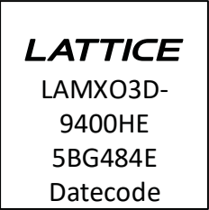
Figure 5.2. Top Markings for Automotive Grade Devices
