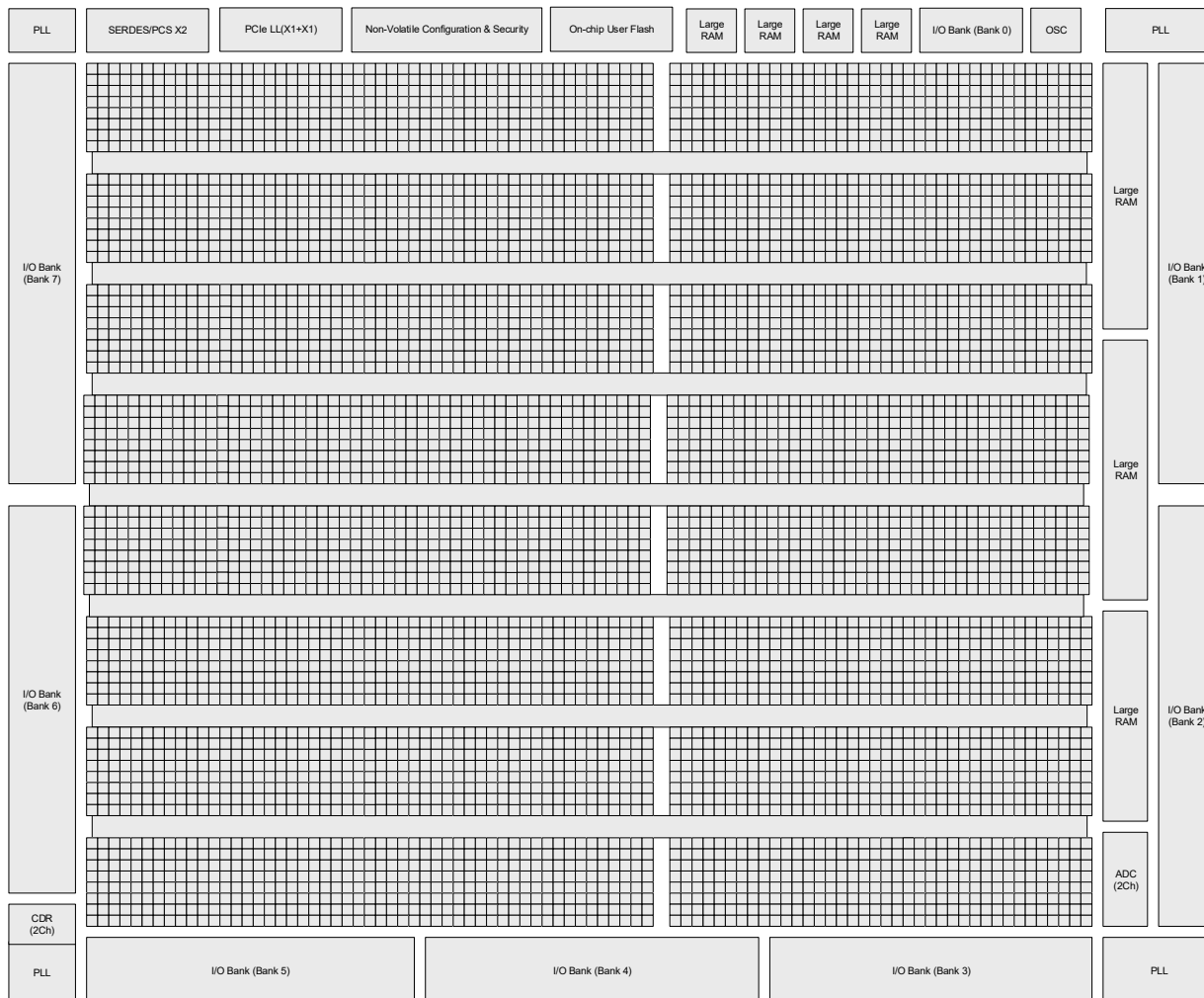
Figure 2.2. Simplified Block Diagram, MachXO5-NX-55T Device (Top Level)
