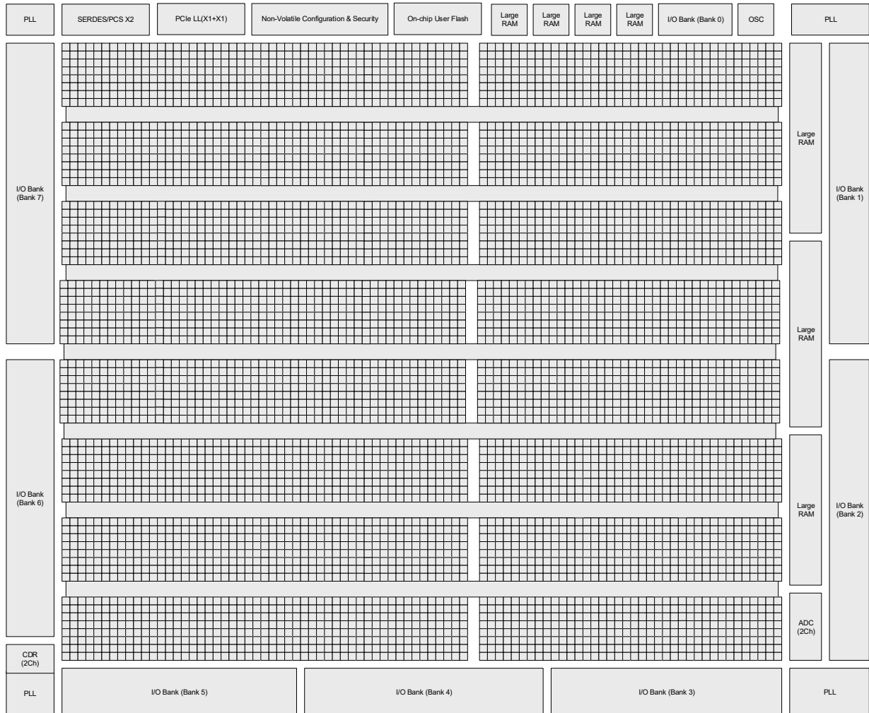
Figure 2.3. Simplified Block Diagram, MachXO5-NX-100T Device (Top Level)
