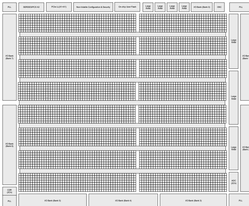
Figure 2.2. Simplified Block Diagram, LFMXO5-55TD, LFMXO5-55TDQ, LFMXO5-55TDQE, and LFMXO5-65TDQ Devices (Top Level)
