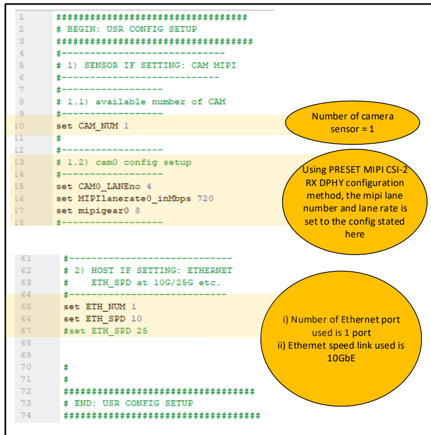
Figure 4.17. Required PDC Configuration
